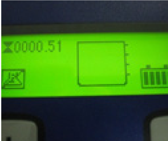
1. Check battery charge gauge.
